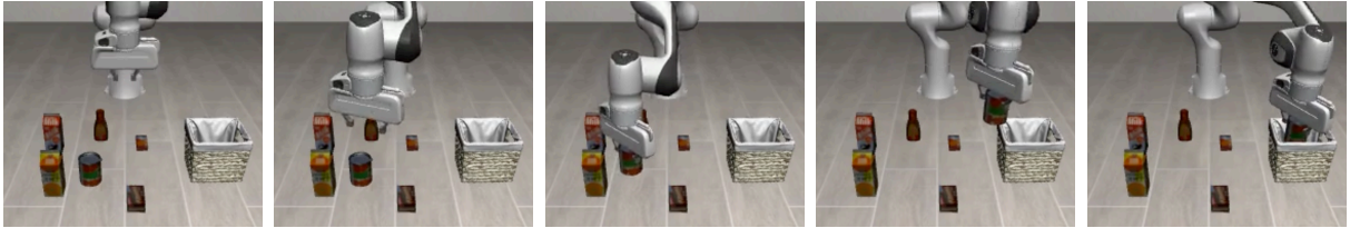
Figure 7: Data Selection Qualitative Result. In the first video, the robot grasps the wrong object, which is the cream cheese. In the second, the robot moves toward the ketchup but knocks it off before moving to the basket. The robot successfully completes the task in the third video.
