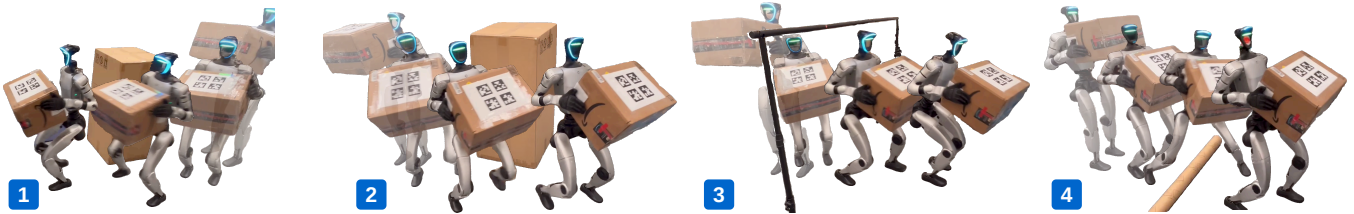
Fig. 1: We introduce HOTICE , a humanoid loco-manipulation method that enables humanoid robots to transport objects through cluttered environments populated by diverse types of obstacles, including side obstacles – (1) and (2), overhead obstacles – (3), and ground obstacles – (4). More results can be found at our anonymous website https://hotice2027.github.io .
